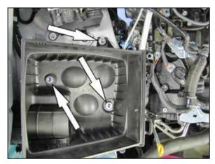
7. Remove the three bolts securing the lower air filter housing to the inner fender and then remove the lower air filter housing from the vehicle. NOTE: K&N Engineering, Inc., recommends that customers do not discard factory air intake.
