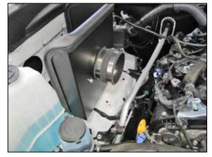
14. Install the provided coupler (08698) onto the filter adapter and secure with the provided hose clamp.
