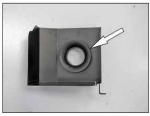
10. Install the provided radius adapter onto the heat shield and secure with the provided hardware.
