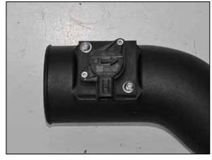
18. Install the mass air sensor assembly into the K&N $^{\circ}$  intake tube and secure with the provided hardware.
