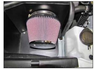
23. Install the K&N® air filter onto the filter adapter and secure with the provided hose clamp. NOTE: Drycharger<sup>®</sup> air filter wrap; part # 22-8049DK is available to purchase separately. To learn more about Drycharger® filter wraps or look up color availability please visit http://www.knfilters.com®.
