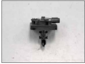
17. Install the mass air sensor into the adapter and secure with the provided hardware.
